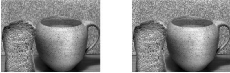
Fig. 4. Original images: near focused (left); far focused (right). The difference between the two images is barely perceptible since the two focal planes are only 340 mm apart.
