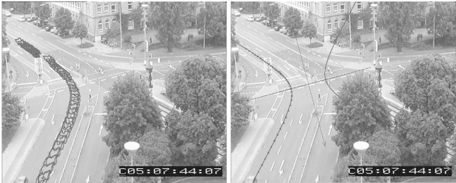
Fig. 3. Left panel: The OIC-mask contours, shown every 20 half-frames, with small dark ‘x’ denoting the center of an OIC-Mask. Right panel: The ‘lane spine’, a hyperbola fitted according to equ. 1 – using every half-frame – to the OIC-mask trajectory shown in the left panel.
