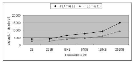
Fig. 7. MPI\_Bcast with different message sizes.
