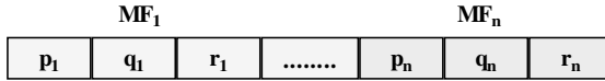
Fig. 5. Chromosome representing n MF for every input/output variable coding the parameters of a bell shape MF
