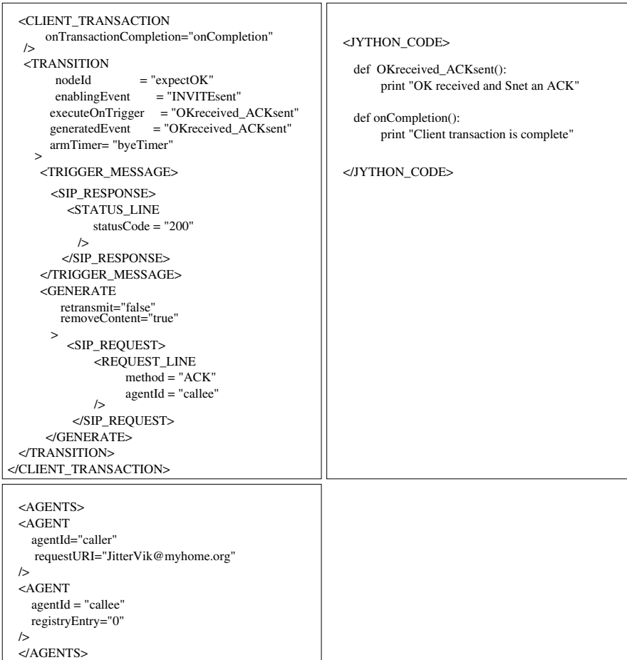
Fig. 4. A Call Flow is represented as a set of TRANSACTIONs Events TIMERs and triggered TRANSITION nodes. TRANSITIONs are triggered by events and messages can generate outgoing messages and events to trigger other Expect Nodes. An AGENT is a short hand way of referring to a user identity. An AGENT entry can refer to a registry entry in the Proxy server. This is bound at run time to an actual value (see Section 5).
