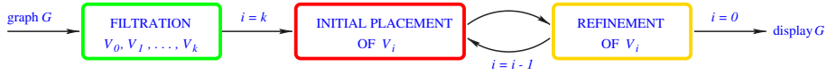
Fig. 1. An overview of the algorithm. Given a graph G , the algorithm proceeds phases. The first phase creates a MIS filtration. The second and third phases use the filtration sets V_k, V_{k-1}, \dots, V_0 to repeatedly add more vertices and refine the drawing.
