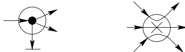
Fig. 1. An active node (left) with an in-degree of 1 and an out-degree of 2 as well as a passive node (right) with an in- and out-degree of 3.
