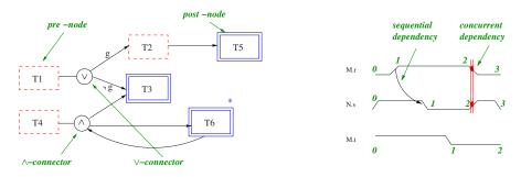
Fig. 3. A Modular Timing Diagram and a component RTD
