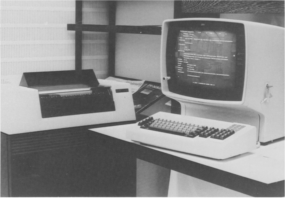
FIG. 9: INTERACTIVE INPUT/OUTPUT TERMINAL: IBM 3270
