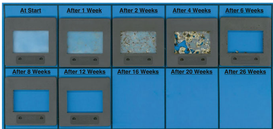
Fig. 21 Disintegration test under 28°C (referring to ISO 20200) by OWS. Specimen: 111 μm thickness film of developing grade
