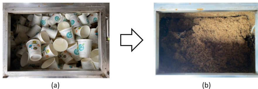
Fig. 19 Composting test of PBS coated paper cup. (a) PBS coated paper cups were mixed with the substrate in the composting machine. (b) Almost no residues of paper cup were observed after 24 h treatment
