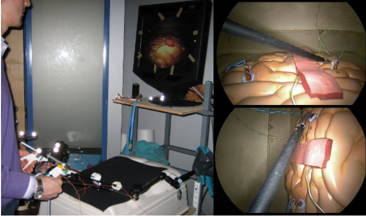
Fig. 1. (a) Experiment setup showing the arrangement of the IR sensors in relationship to the laparoscope tools, and the plastic small bowel model with a simulated omental flap with and without the camera view being rotated (b-c)
