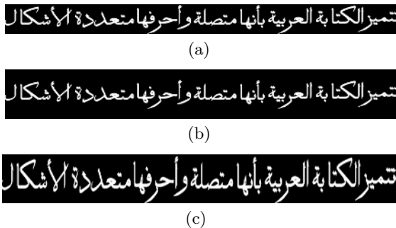
Fig. 7. Text lines with different line heights: (a) 43 pixels, (b) 60 pixels and (c) line image in (a) resized to 60 pixel size
