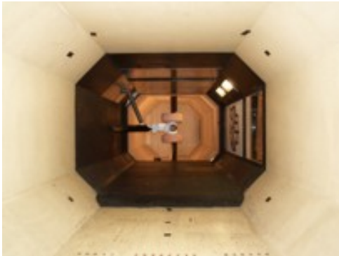
(a) Aircraft landing-gear test in wind tunnel using microphone arrays
