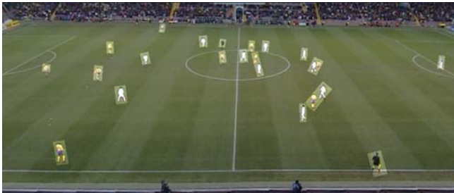
Fig. 3. The set of ellipses, \mathcal{E}_t , the highlighted regions, found by background subtraction
