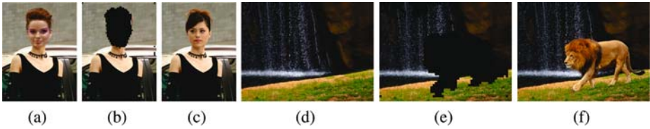
Fig. 1. Examples of image doctored and our detection results. (a) and (d) are two doctored JPEG images, where (a) is synthesized by replacing the face and (b) is by masking the lion and inpainting with structure propagation [9]. (b) and (e) are our detection results, where the doctored parts are shown as the black regions. For comparison, the original images are given in (c) and (f).
