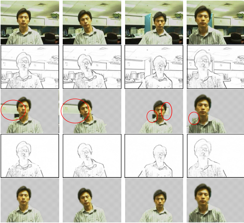
Fig. 3. Background contrast attenuation. Top row: several frames from a video. Second row: contrast maps. Third row: segmentation results by the basic model. Red circles indicate notable segmentation errors. Fourth row: attenuated contrast maps. Last row: segmentation result using attenuated contrast map.
