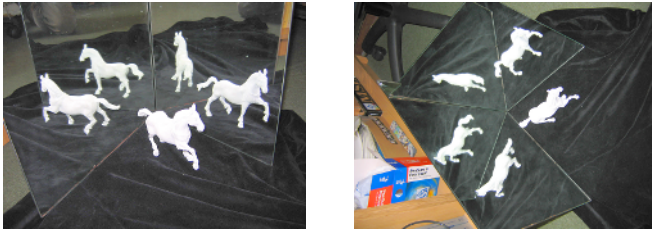
Fig. 1. Two images of a double mirror setup positioned so that five views of the object can be seen. Note that the camera has moved between shots, but the mirrors and object have not moved.
