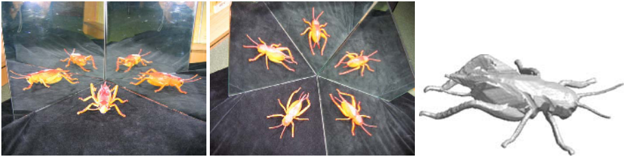
Fig. 7. Two input images and resultant visual hull model of a toy locust
