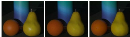
Fig. 4. Comparison to ground truth. Left: input image. Center: ground truth diffuse component obtained using linear polarizers. Right: diffuse component recovered using anisotropic multi-scale erosion.
