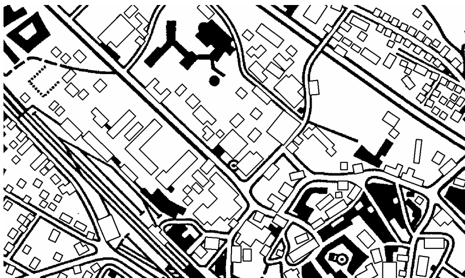
Fig. 7. A fragment of the city map from Fig. 1 with borders of orthogonal buildings (the result of processing by ArcScan for ArcGIS)
