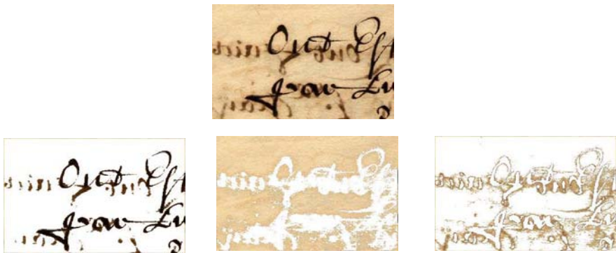
Fig. 2. Results of the 3-means classification algorithm on a degraded image; Top: An extract of a degraded document image; Bottom: Left: Image class n^{\circ}1 , Middle: Image class n^{\circ}2 , Right: Image class n^{\circ}3
