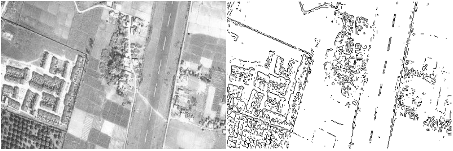
Fig. 7. (a) Original contaminated image. (b) Edge detection using proposed method.
