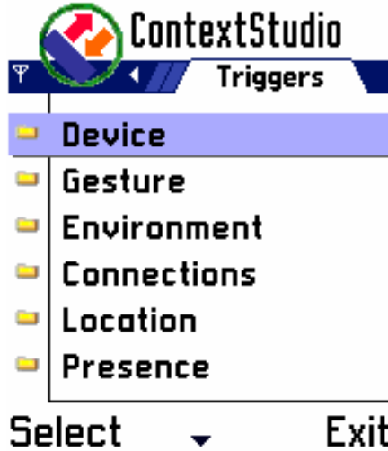
Fig. 2. The folder structure in the triggers view. The folders describe the attribute type and can contain subfolders, which the user can navigate to find the desired attribute value.
