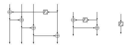
Using this framework we can define key schedules for the small scale variants. SR(n,r,c,e) has a user-provided key of size rce bits, which is considered to be an array of  $(r \times c)$  e-bits words. This key forms the initial subkey. Each subkey is then used to define the succeeding subkeys. We provide a full description of the small scale key schedules in Appendix A.
