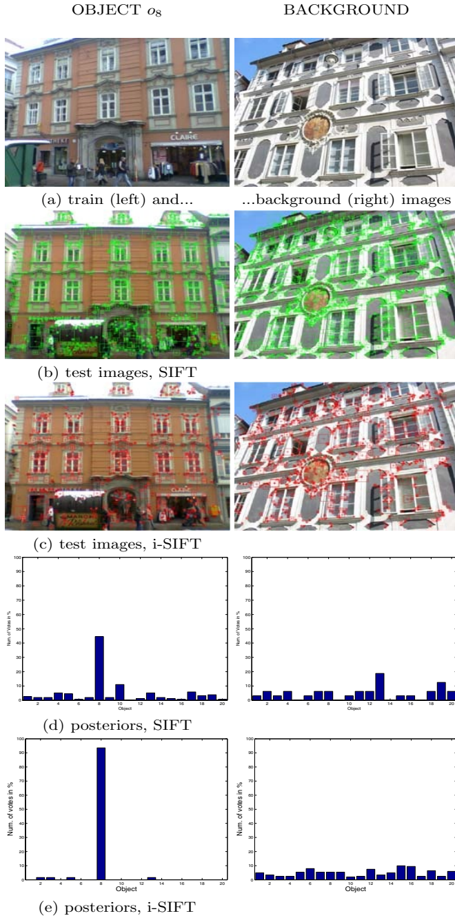
Fig. 4. Sample object detection results for object o_8 (left) and background (right), (a) depicting train images, (b) SIFT descriptor locations on test images, (c) selected i-SIFT descriptors, (d) posterior distribution on object hypotheses from SIFT and (e) i-SIFT descriptors, demonstrating more distinctive results for i-SIFT based interpretation
