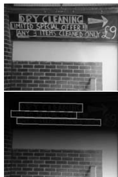
Fig. 1. Text detection based on category-specific extremal regions
