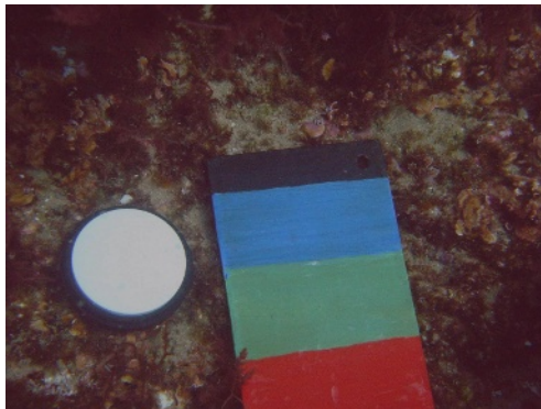
Fig. 7. Corrected image with new K_d value for the red channel
