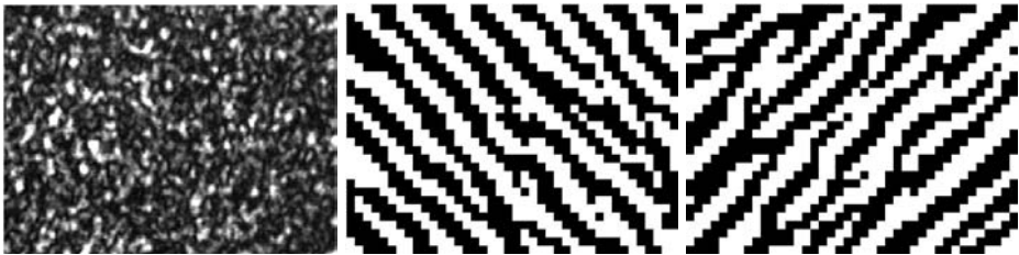
Fig. 3. Left: Example of a speckle pattern. Middle: Binarized Gabor coefficients at 45°. Right: Binarized Gabor coefficients at 135°.
