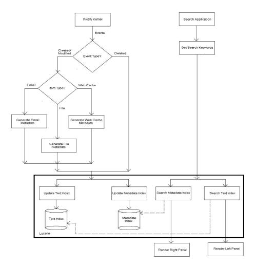
Fig. 5. Prototype Application Architecture
