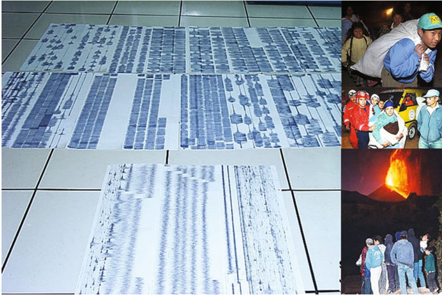
Fig. 6 Left Seismograms of the December 2000 activity ( back ), showing highly saturated recordings, compared with seismicity recorded for the largest previous eruptive event in June 1997 ( front ), which caused ashfall on
