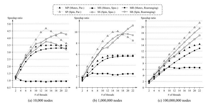
Fig. 3 Speedups in the case of one 24-thread Xeon, 8-node task
