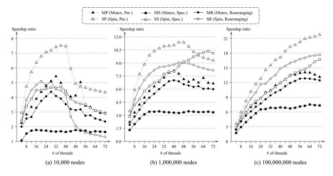
Fig. 6 Speedups in the case of POWER8, 8-node task
