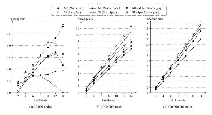
Fig. 16 Speedups in the case of M1 Ultra, 64-node task
