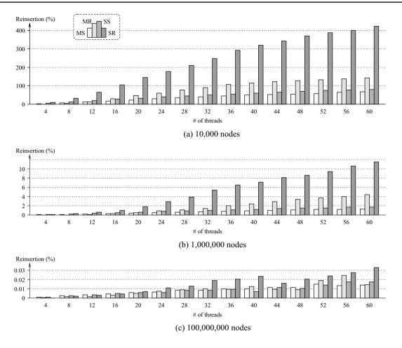
Fig. 5 Reinsertion ratios in the case of two 32-thread Xeon's, 8-node task
