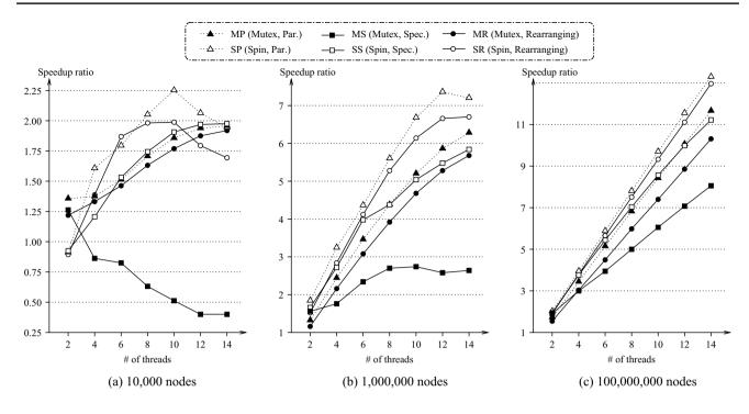
Fig. 8 Speedups in the case of M1 Ultra, 8-node task
