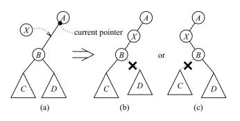
Fig. 1 Example of restructuring the BST on the node insertion
