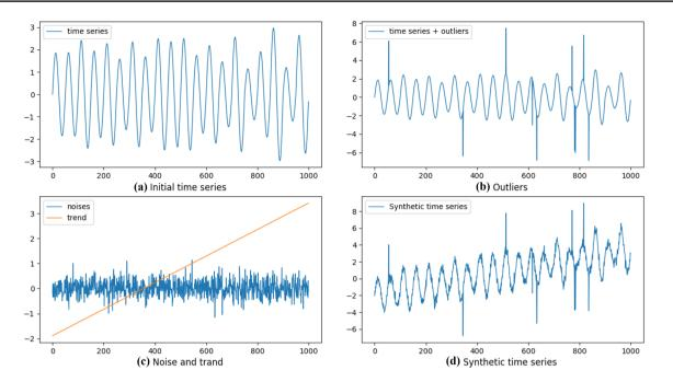
Fig. 7 The generation of synthetic data. **a** Create a time series consisting of sine waves with randomly varying amplitude; **b** Add random outliers; **c** Generate random Gaussian noise and trend; **d** Add noise and trend to generate synthetic time series
