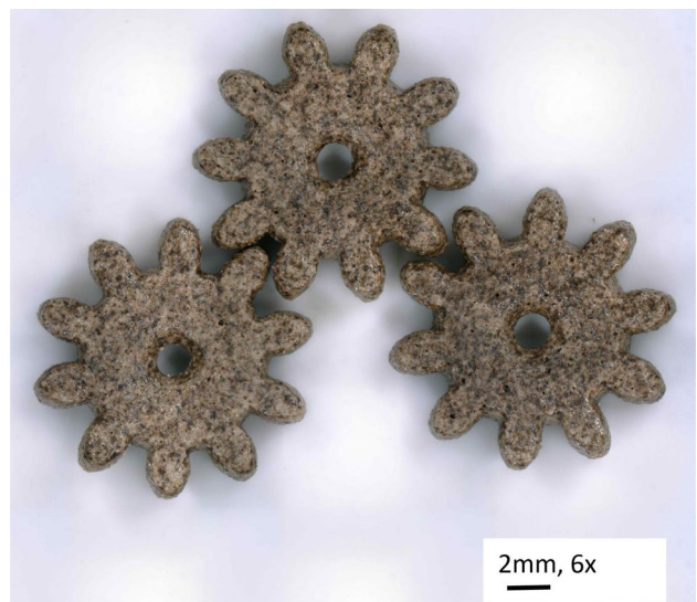
Fig. 1 Example of detailed lightweight and high-temperature printed parts based on hollow ceramic spheres
