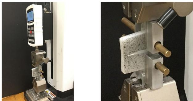
Fig. 2 Experimental setup for compact tension test
