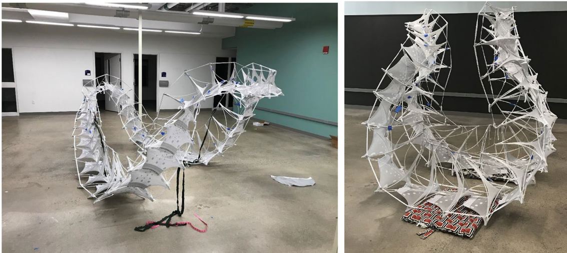
Fig. 18 Equilibrium condition achieved through pre-tensioned knit bands
