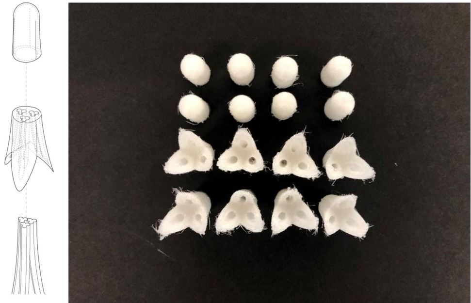
Fig. 13 Design and fabrication for connectors
