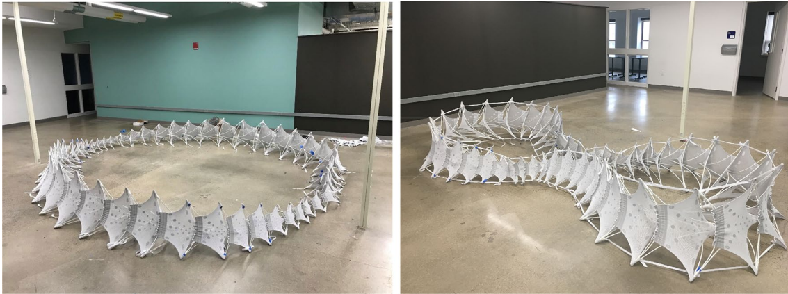
Fig. 17 Tetrahedrons connected into a circle
