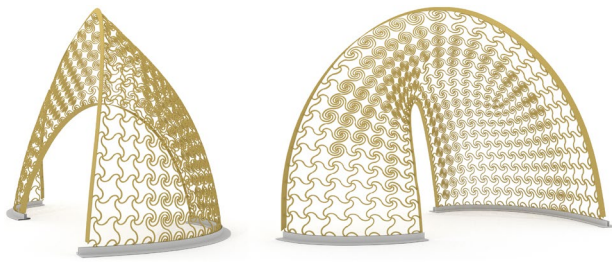
Fig. 5 Preliminary design overall view of the assembled plywood FlexMaps Pavilion. The metal base profile has been later replaced by an all-plywood base in the definitive design. Additionally the twist range of the spirals has been restricted to accommodate milling tolerances
