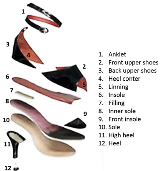
Fig. 2 Footwear components, model of sandal [26]
