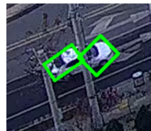
Fig. 16 The video image of a vehicle occluded by a roadside obstruction
