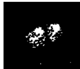
Fig. 15 The binary image of a vehicle occluded by a roadside obstruction
