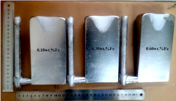
Fig. 1: Experimental wedge castings of Al-6Si-xFe (x=0.10, 0.35, and 0.60wt.%) alloys
