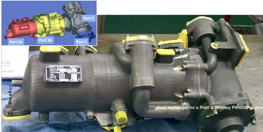
(a) SLS made polyamide-based models of heat exchanger for a Pratt & Whitney PW6000 engine [13]
