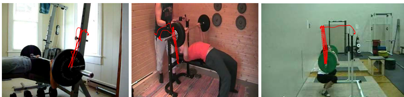
Fig. 6 Examples of load tracking. The motion of the load during each video is overlaid as a red line on a typical frame from the video
