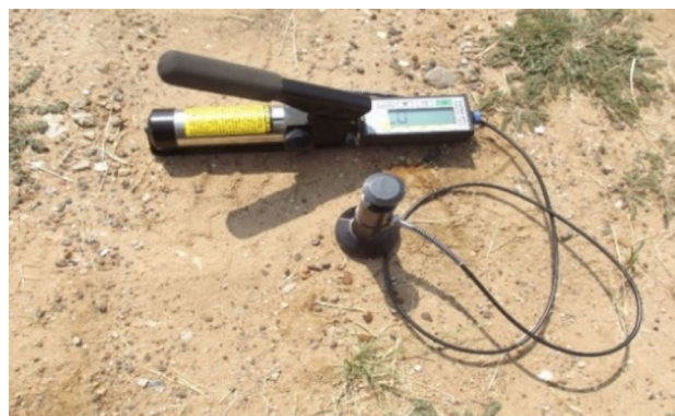
Fig. 3 ASTM pull-off testing apparatus
