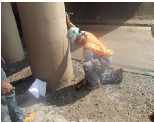
Fig. 5 Pull-off testing procedure
