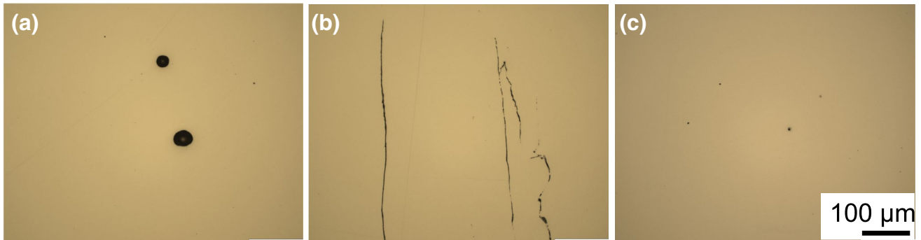
Fig. 3 Optical micrographs of SEBM processed 42CrMo4 powder with the following parameters: a 2 J/mm 2 , 300 W, b 2 J/mm 2 , 900 W, c 3 J/mm 2 , 600 W (build direction is vertical)
