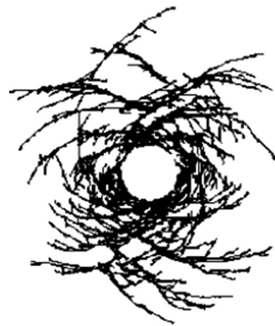
Fig. 14 Further optimization fracture characteristics of tunnel
