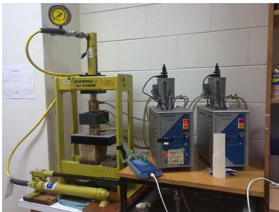
Fig. 5 Divided bar instrument for thermal conductivity measurement
