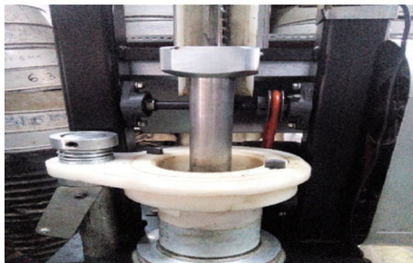
Fig. 8 Compaction of a Marshall specimen in progress
