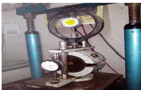
Fig. 10 Marshall test of a DBM sample in progress
