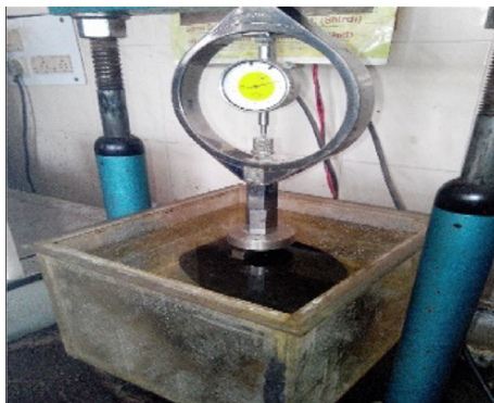
Fig. 13 Moisture susceptibility test in progress
