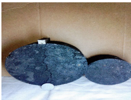
Fig. 14 View of cracks in DBM sample after failure
