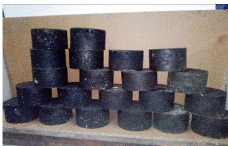
Fig. 9 A view of DBM samples before Marshall testing
