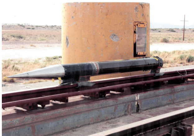
Fig. 1 Picture of a June 2014 HHSTT sled featuring treated 4130 steel slippers on a 1080 steel track rail, obtained from correspondence with HAFB
