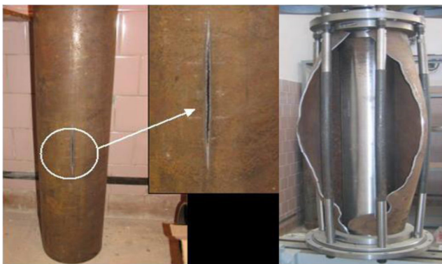
Fig. 2 Rupture initiated from a gouge or/and dent
