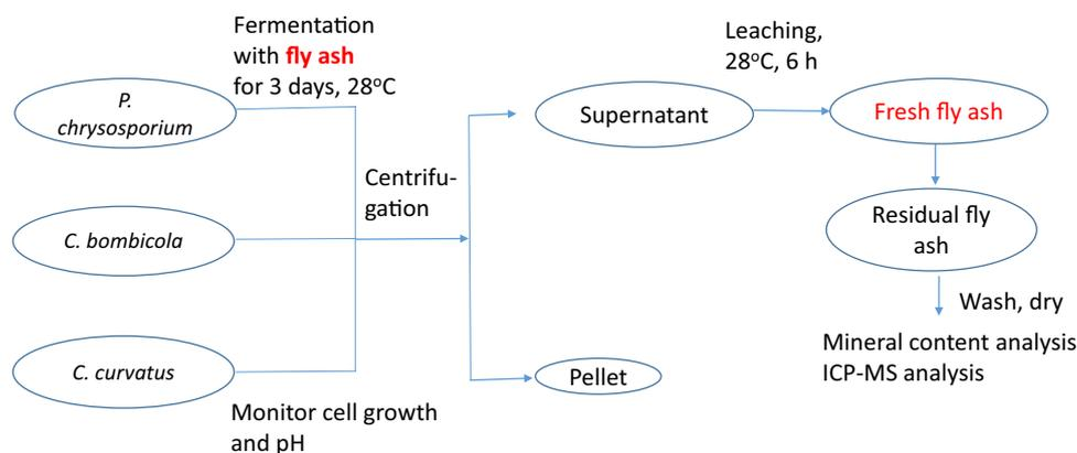
**Fig. 1** The overall experimental design
