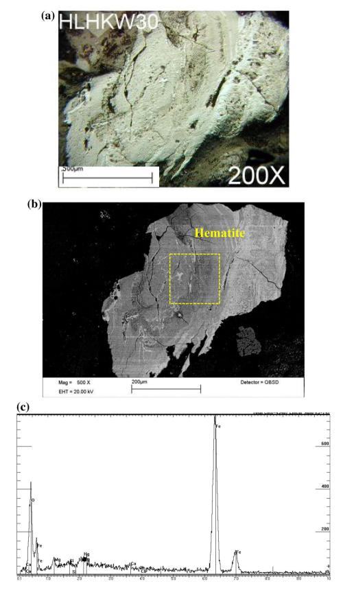
Fig. 4 Hematite in the Huolinhe coal. a Optical microscopy, reflected light; air; polarized light;  $200 \times .$  b SEM backscattered electron image. c X-ray energy spectrum diagram of box in b, scanning area:  $150 \ \mu m \times 150 \ \mu m$
