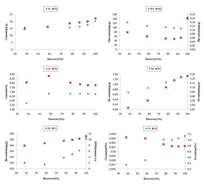
Fig. 8 Washability curves for trace elements in the No.14 coal from the Huolinhe mine
