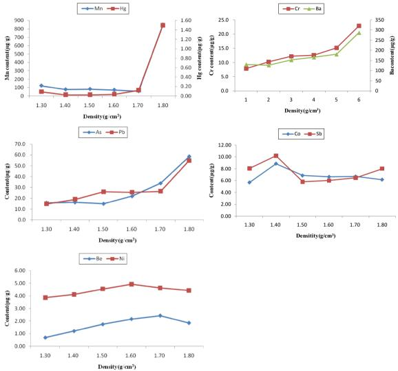
Fig. 7 Variations of trace element concentrations for the products of different densities of the No.14 coal in the Huolinhe mine
