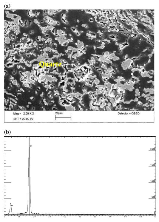
Fig. 2 Quartz in fusinite lumens. a SEM backscattered electron image. b X-ray energy spectrum diagram, spot scan
