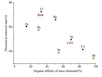
Fig. 9 Relationship between organic affinity and theoretical trace element removal rate in the No.14 coal from the Huolinhe mine
