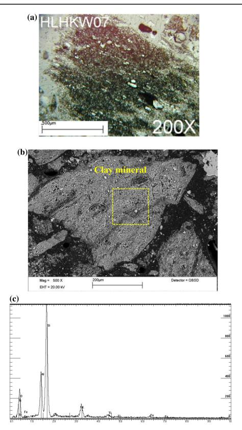
Fig. 1 Clay minerals in the Huolinhe coal. **a** Optical microscopy, reflected light; air; polarized light; $200 \times .$  **b** SEM backscattered electron image. **c** X-ray energy spectrum diagram of the box in **b**, scanning area: 150  $\mu$ m  $\times$  150  $\mu$ m
