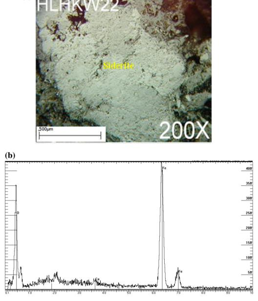
Fig. 3 Siderite in the Huolinhe coal. **a** Optical microscopy, reflected light; air; polarized light; $200 \times b$  X-ray energy spectrum diagram scanning area: 100  $\mu$ m  $\times$  100  $\mu$ m
