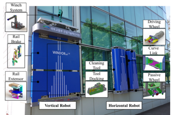
Fig. 2 Components of building façade maintenance robot
